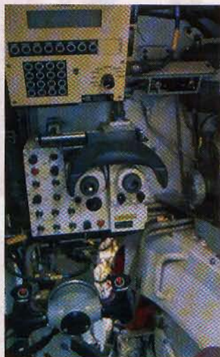
Gunner's day-and-night sight and yoke; steering wheel, brake (centre) and accelerator pedal - easy
