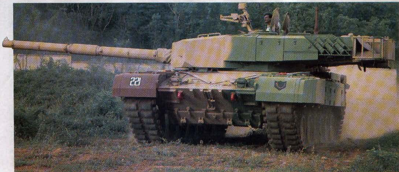
The turret 'floats up' when in stabilised mode; the 120mm gun can slew through 90 degrees in just two seconds and fire on the run.
