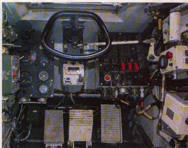
Gunner's day-and-night sight and yoke; steering wheel, brake (centre) and accelerator pedal - easy
